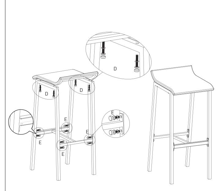
Attach support bar(B) to legs (A) with using bolts and washers(E).
