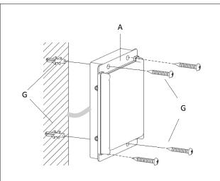
Drill four holes in the wall using the holes in the fitting body 'A' as a template. Use screws and suitable fixture system 'G' to install the fitting 'A' onto the wall securely. NOTE: The fitting can be installed in any orientation. Always ensure that grommet' F' is tight around the cable and it is not damaged. Apply silicone if required to maintain IP rating.
