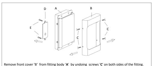
Remove cover 'D' on the back of the fitting by undoing 2 x screws 'E' to access the terminal block .
