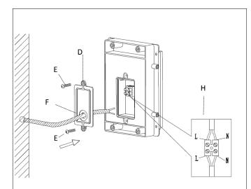
Feed mains supply cable through the wall and weatherproof grommet 'F' of the cover 'D'. Ensure grommet seals well. Apply silicone if required to maintain IP rating.
