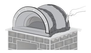
Using your trowel, place strips of bonding cement around the base of the oven and in between the external joints of the three chambers.
