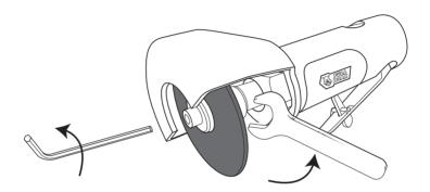
4. Ensure the cutting disc is correctly mounted and tightened before use and run the tool at no-load speed for at least 1 min in a safe position; stop immediately if considerable vibration or other defects are detected and determine the cause of the defects and remedy these defects before use.
