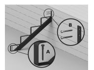
A: Attach bottom of each stringer using M10 x 50 mm coach screws\* for timber, or M10 x 60 mm Ramset™ WERCS Ankascrew™ anchors for concrete.
