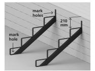
Determine the location of all stringers and ensure the top tread support is 210 mm down from upper deck surface. Then, for each stringer, level and mark the two fastener locations on the deck rim, and one fastener location on the lower deck surface.
