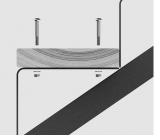
3 Install each timber tread using M8 x 60 mm cup head bolts, nuts and washers.
