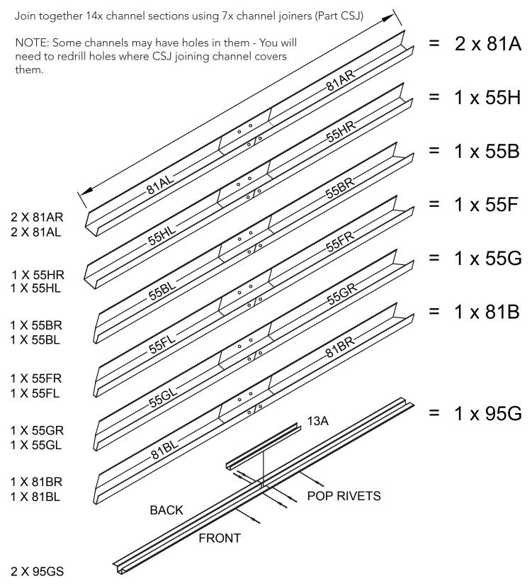
NOTE: Channels 55G, 55F, & 55H are best secured together using pop rivets through the 15mm high (front) edge. This minimizes interference with the sliding doors
