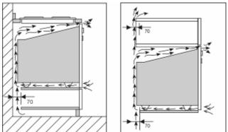
The unit panels next to the cooker must be heat resistant. In the case of veneered wood units, glues must be resistant to a temperature of 120°C.
