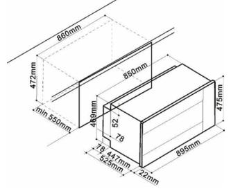
To provide adequate ventilation, there must be appropriate ventilation opening, the panel to which the oven is fitted should have a gap of at least 70 mm at the rear.
