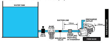
WARNING! The input hose or pipe should be low enough in the water to ensure that if the water level falls, the pump will not run dry. Ensure that this is checked when in operation.
