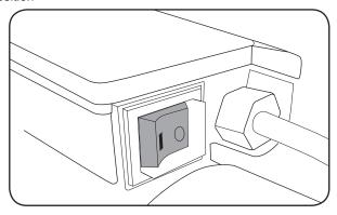
3. To turn the pump off, depress the ON/OFF switch to the OFF (0) position.
