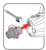
Securely attach the input hose or pipe to the other end of the adaptor. Ensure you have the correct diameter hose or pipe that is compatible with your water drawing source.
