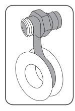
Remove the plastic protection cover from the suction inlet and insert a 1" male threaded hose adaptor (not included). Tighten firmly with a spanner (not included).
