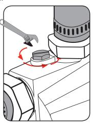
Using a hose, fill the pump completely with water. Ensure the pump and inlet pipe or hose are full. Replace the priming screw.
