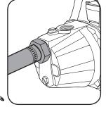
**NOTE:** The input hose or pipe you are using must have a minimum diameter of 25.4mm (1").
