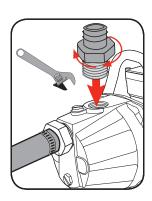
3. Securely attach the output hose or pipe to the other end of the adaptor. Ensure you have the correct diameter hose or pipe that is compatible with your water discharge application.
