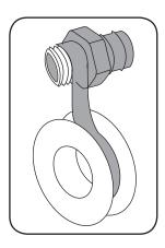
Remove the plastic protection cover from the discharge outlet and insert a 1" male threaded hose adaptor (not included)..
