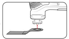
3 Replace the washer and accessory locking bolt.
