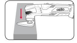
**Note:** Do not apply heavy pressure to the tool or tilt the sanding base as this will wear out the sanding paper and may damage the sanding pad.
