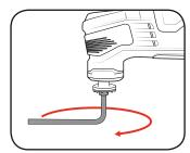
2 Place the desired accessory onto the accessory drive spindle ensuring the holes in the accessory align with the notches on the tool.
