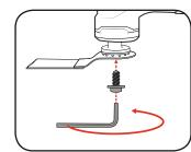
4 Pull on the accessory to check if it is secured correctly.
