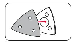
3 To remove, peel away from the sanding pad starting from an edge.
