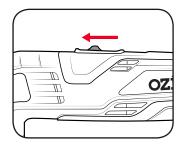
Place the multi function tool flat on the workpiece and make smooth back and forth movements
