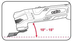
**Note:** Allow the scraper to do the work, do not apply heavy pressure to the tool. This may cause the multi function tool to overload or cut into the surface of the material.
