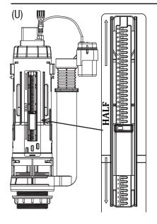
For 3L Half Flush, set the Half Flush Adj. to 21. If the slider is higher, less water will be released.
