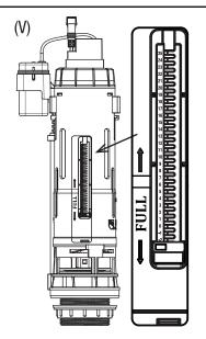
For 6L full flush, set the large Full Flush Adj. to digit -2. For 4.5L full flush, set to digit 2.
