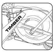
**Note:** A piece of timber will assist in holding the blade while removing or tightening the blade bolt.
