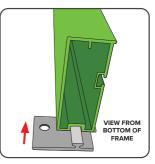
Starting from the bottom of one frame side, slide 4x brackets into the track (as shown above).
