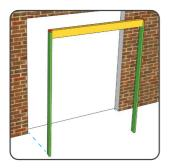
Position constructed frame into door opening. Ensure frame is square and level. Spin frame to set left/right operation (i.e. Having the hinges/door connector clips on the left will mean door will close from left to right).
