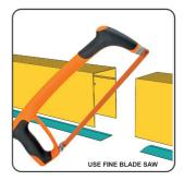
Door width can be altered to suit opening. Measure and trim headrail and bottom rail as required.
