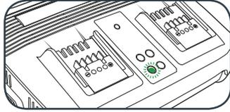
3. Align and then slide the ribs on the battery into the recess in the charger.
