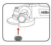
6 Depress and hold the spindle lock button. Firmly tighten the outer flange with the pin spanner.
