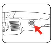
2 Press the on/off trigger to start the grinder.
