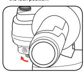
3 Use the pin spanner to loosen the outer flange.
