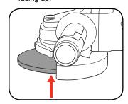
5 Screw the outer flange onto the spindle.
