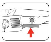
4 Begin grinding your workpiece. The optimum grinding angle is 10-15° to the workpiece. Do not apply excessive pressure. Allow the tool to do the work. This will prevent deep gouging.
