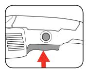
3 To stop the grinder, release the on/off trigger.
