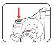
2 Rotate the spindle to locate the lock position.
