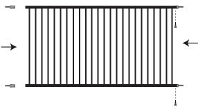
Insert fixing brackets into pool fence panels (panels sold seperately) as shown and fix off with screws.
