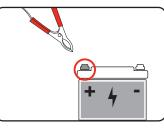
2. Connect the black negative terminal clamp to an unpainted piece of metal on the bodywork away from the battery.
