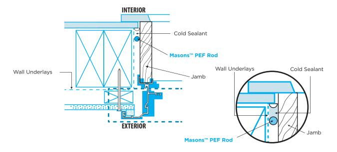
• Cut the PEF Rod to the required length and press the into the gap with a blunt tool to provide an even depth, avoid stretching and twisting the PEF Rod.
