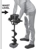
CORRECT OPERATING POSITIONS IS WITH POST HOLE DIGGER HANDLES BELLOW WAIST LEVEL
