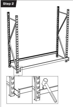
Attach Beams 'B' to each Upright 'A' using the bottom keyholes and tap into place using a rubber mallet.
