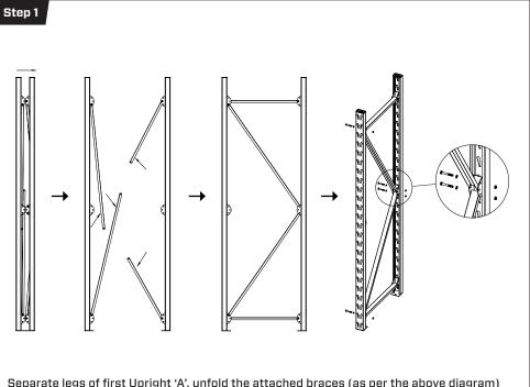
Separate legs of first Upright 'A', unfold the attached braces (as per the above diagram) and fix the legs together using the provided Bolts and nuts 'F'. Please note: washers should be positioned either side of each brace. Repeat above steps for second upright.
