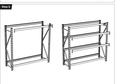
Repeat this step using two Beams 'B' for the top keyholes. Then attach the remaining beams at your desired heights, tapping them into place with a rubber mallet.
