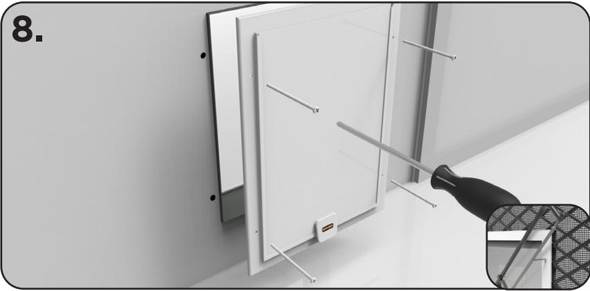
8. Screw inner door frame into door/panel. Tighten with a Phillips headscrew driver. If screws protrude, trim using a hacksaw.
