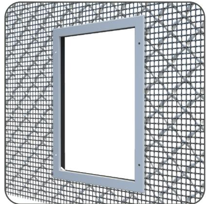
3. Fit all 4 partitions into outer door frame, use duct tape to secure the corners then place into opening. If the security screen has insect mesh, place a bead of construction silicon around the internal section of the pet door and on the mesh surface. Apply this around the cut out in order to hold the mesh in place when both frames are joined.
