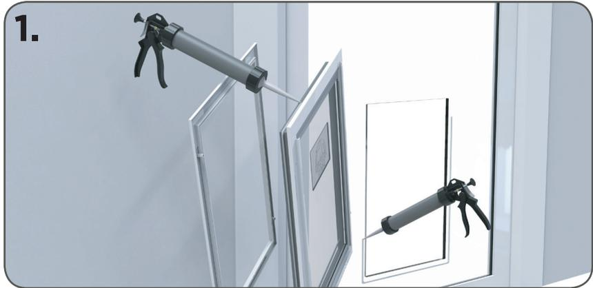
1. Refer to steps 1 and 2 of “Installation”. **IMPORTANT:** Contact a professional glazier to cut out the opening for the pet door. Place a bead of construction silicon around the internal section of the pet door and on the surface around the cut out to provide a weather seal. Note the tunnel partitions will need to be cut to size as per step 6 of “Installation”.
