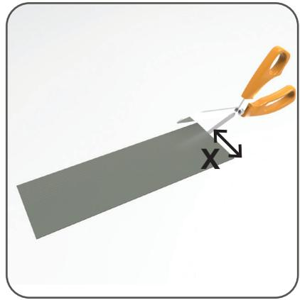
6. Measure the thickness of the door/panel and add 10mm(3/8") (x) so the tunnel protrudes 5mm(3/16") on each side. If required, cut partitions down to correct size.
