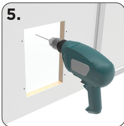
5. Insert outer frame into opening and mark screw holes. Drill each of the screw holes using a 8mm(5/16") drill bit.
