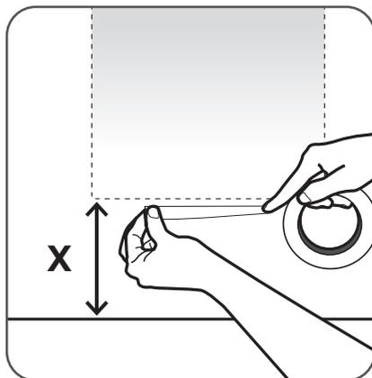
1. Measure the height (x) from the underside of the dog's stomach to the floor. Mark height (x) on door/panel with tape or similar.
