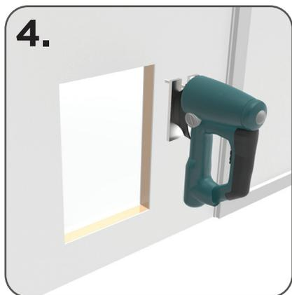
4. Using a reciprocating jigsaw, cut out the opening, cutting along the pencil outline.
