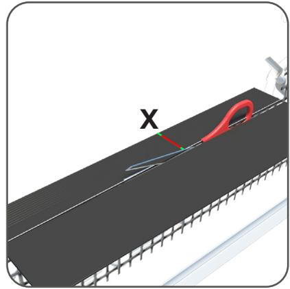
2. Measure the thickness of the door/panel and add 10mm(3/8") (x) so the tunnel protrudes 5mm(3/16") on each side. If required, cut partitions down to correct size.
