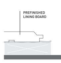
Place first lining board on batten/surface with tongue facing outwards.
