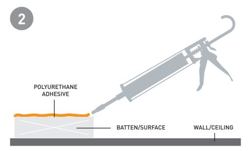
Apply polyurethane adhesive to batten/surface.
