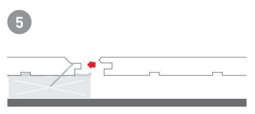
Slide in next lining board and continue with adhesive and nailing until you have lined your surface.
