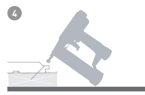
Nail through the protruding tongue on a 45-degree angle.
