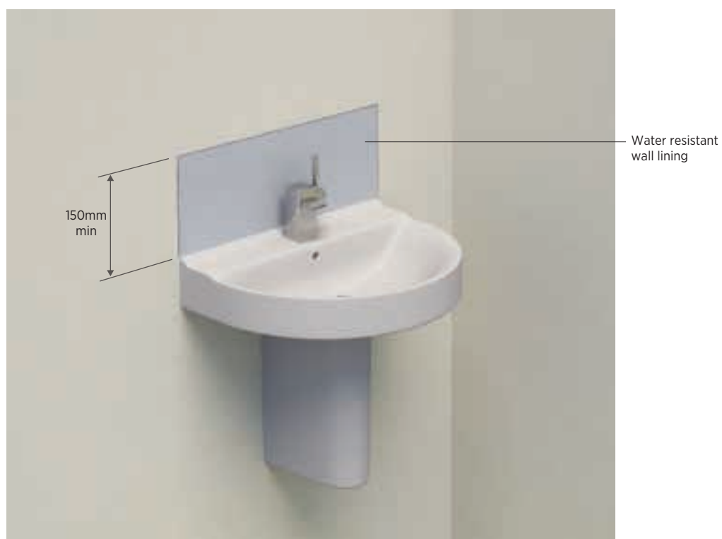
Figure 58: Waterproofing of basin
