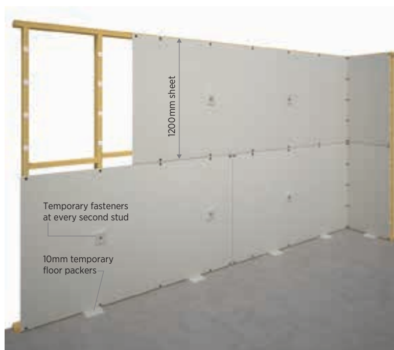
Figure 29: Combination adhesive and screw fixing on walls
