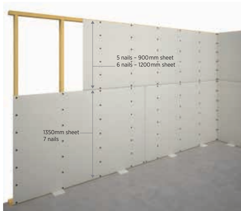
Figure 31: Nail fixing to walls (single nails)
