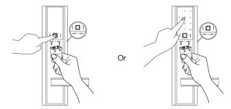
While connecting a 9-V battery to the external power (emergency battery) contact point on the outer body, place a recognized fingerprint or enter a password.
