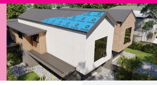
SilverSark® xR is a Heavy Duty double-sided radiant barrier, designed for use under metal deck roofs where temperatures can exceed 80°C, and with battened out cladding to create an extra reflective air space for enhanced R-value. It is an Air and Water Barrier, Class 2 Vapour Barrier product, suitable for use in all roof and wall applications.
