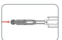
2 Make sure that the rotation direction indicated by the arrows on the belt and the tool match.
