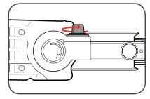
2 Adjust the angle of the rotating file arm to the desired position.
