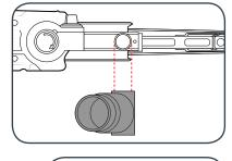
2 Press the dust adaptor onto the rotating file arm so that the tabs on the adaptor clip over the arm.
