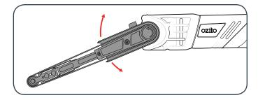
3 Secure in place by rotating the rotating arm screw clockwise.
