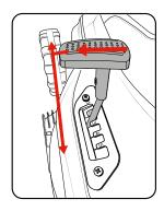
WARNING: BE CAREFUL DURING CUTTING HEIGHT ADJUSTMENTS OF THE LAWN MOWER TO PREVENT ENTRAPMENT OF THE FINGERS BETWEEN MOVING HEIGHT ADJUSTMENT LEVER AND THE MOWER HOUSING.
