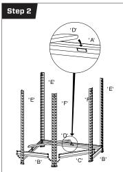
Use two shelf brackets 'B' for the side brackets using the shelf bracket from Step 1 as a guide for height, followed by shelf bracket 'C' as shown in the diagram. Place brace 'D' as shown.
