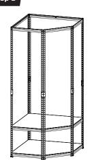
Repeat step 4 for remaining shelves. We recommend working from the bottom up, this will make placing the MDF shelves in easier.
