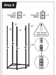
the connector plates, as shown in the diagram, taking into account upright position. Note: The legs are designed to sit directly on top of each other don't overlap them.
