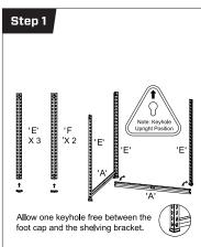
Place footend caps onto the bottom of the 5 legs 'E' and 'F'. Note upright position. Place shelving bracket 'A' onto the legs. A rubber mallet can be used to lightly tap all brackets into the keyholes on the legs.
