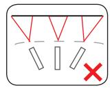
2. Keep the spray gun perpendicular to the surface, so spray distance is consistent.
