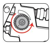
2 Partly tighten the dial then test setting on a scrap piece of material.
