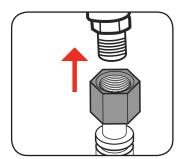
3 Pull back the sleeve on hose fitting, insert male end & release sleeve on hose fitting.
