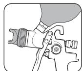
3 Fill paint pot with appropriate cleaning solution.
