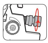
2 Slightly loosen the fluid adjustment dial, then test setting on a scrap piece of material.
