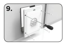
Screw into door from inside. Place nut over screw ends, cut off excess plastic screws. Optional: seal around frame of pet door with silicone.
