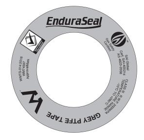
Gas Usage: Applicable Standard: AS 4623-2008 Classification: Class III Rated Working Pressure: 2000 kPa Working Temperature Range: -10°C to +260°C Recommended Application: Suitable for use in metallic threaded joints and fittings used in Natural Gas and Liquid Petroleum Gas (LPG) installations.
