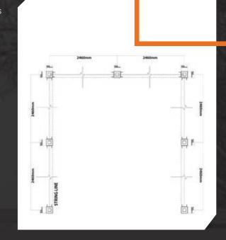
// Make up each of your posts according to step 1 using the 50mm x 50mm square posts and the Panel Channel. Each post is made according to its position in the layout and is either a 180 degree, 90 degree or an end-of-line combination.
