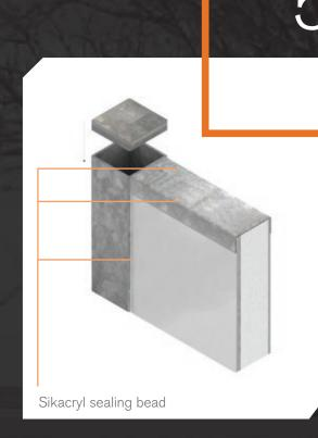
// Prepare the surface of the panels to ensure they are clean and ready to paint. Lightly scuff the metal posts with a scouring pad and ensure they are clean. Use Sikacryl Super (or equivalent) gap sealant between the joins of the Fence Panels to minimize the joint before painting.
