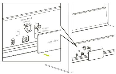
The drawer front can be easily adjusted with the mechanisms on the sides of the drawer. Use the horizontal front adjustment to adjust left and right. Use the vertical front adjustment to adjust up and down.
