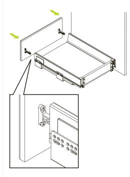
Align the drawer front clips with the drawer sides and push into place.
