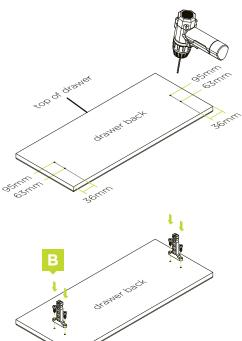
Draw a line 36mm in from each side of the drawer. From the bottom of the drawer mark a point 63mm and 95mm on the lines.
