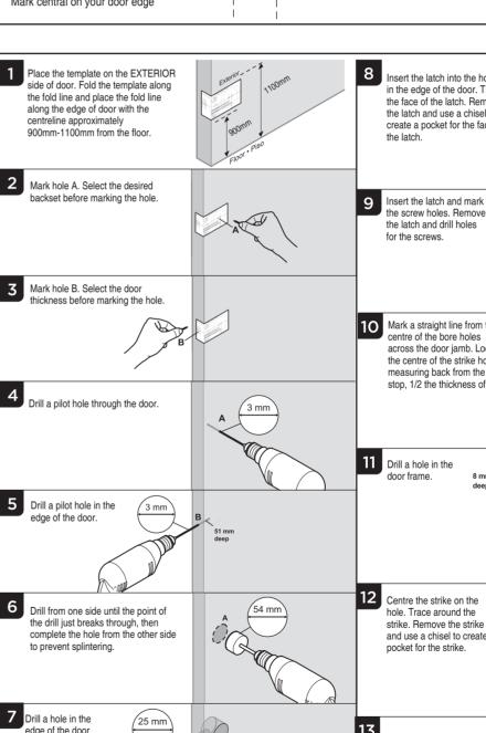
nsert the latch into the hole in the edge of the door. Trace the face of the latch. Remove the latch and use a chisel to create a pocket for the face of
