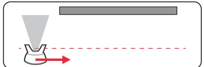
3. Overlap each pass over the workpiece by 2cm to achieve an even coating.
