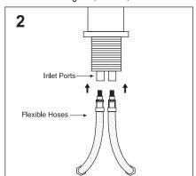
Hand-tighten the flexible hoses into the inlets, being careful to avoid damage to the O-ring seals. If the hoses have red and blue indicators make sure they are connected to the correct inlet ports in the mixer.
