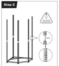
Join the upper and lower legs with the connector pins, as shown in the diagram, taking into account upright position. Note: The legs are designed to sit directly on top of each other – don't overlap them. Handy Hint: Flathead screwdriver may be used to tap in connector pins.
