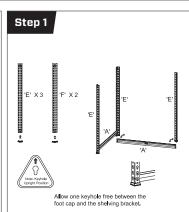
Place foot end caps onto the bottom of the 5 legs (E & F). Note upright position. Place shelving brackets (A) onto the legs. A rubber mallet can be used to lightly tap all brackets into the keyholes of the legs. Allow one keyhole free between the foot end cap and the shelving bracket.
