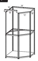
Fix brackets (A, B & C) at the very top allowing room for the MDF board to sit flush against the legs, followed by brace (D) as done previously.
