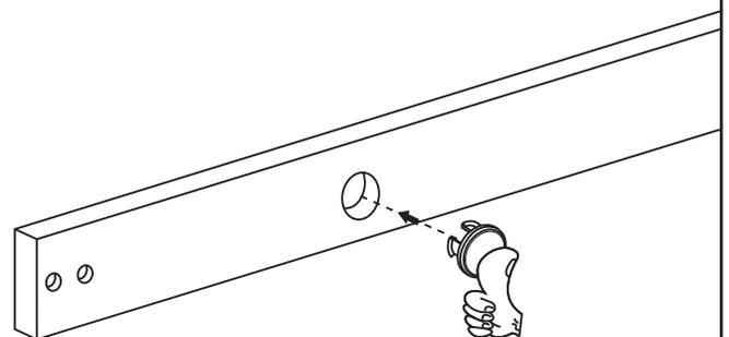
Using the 9mm plastic blanking plugs provided, plug the holes that will not be used to mount the track to the wall.
