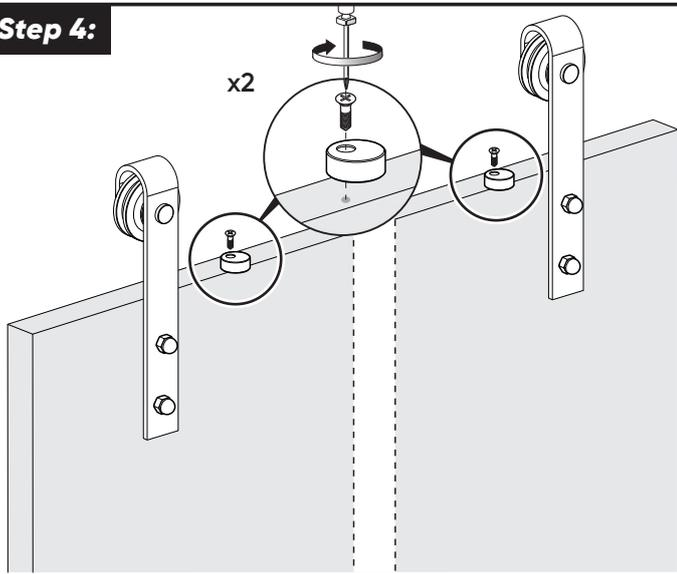
Screw the anti-bounce guide over the edge as shown above. After installing the door, rotate them to fit flush with the door. See Step 5.
