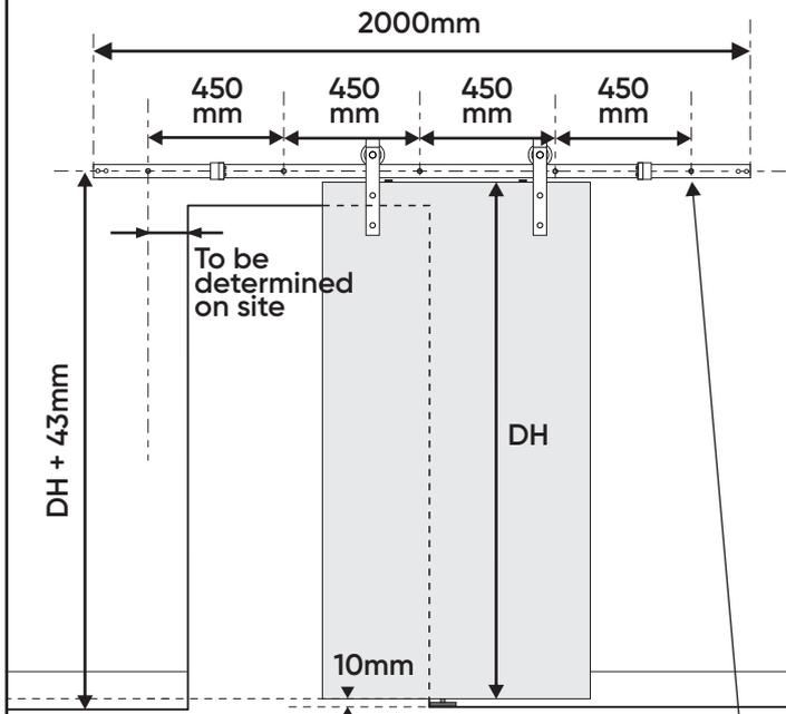
Locate the position of your track. Ensuring the track is level, mark the holes on the wall with a pencil. This will give you a horizontal guide.
