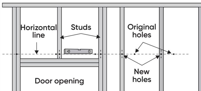
Using a stud finder, fins and mark the centres of the studs along that horizontal line.
