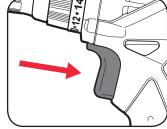
6 Move the drill bit into the workpiece.
