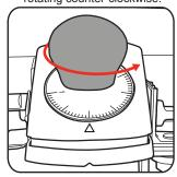
**NOTE:** Set the Depth Adjustment Knob back to '0' once finished with the tool to protect the blades from damage.
