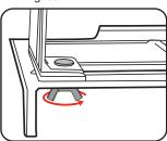
3 Place one of the supplied thumbscrews into the hole and tighten by rotating it clockwise. 2 Align the Angle Bracket with the hole on the side of the planer.
