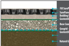
Fill SurePave (STEP 9) SurePave (STEP 7) Bedding Layer (STEP 6) Geotextile - optional (STEP 4) Base Course (STEP 3)
