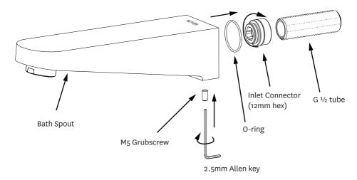
NOTE - Maximum hole diameter through wall for G<sup>1</sup>/<sub>2</sub> tube is 22mm (<sup>7</sup>/<sub>8</sub>")
