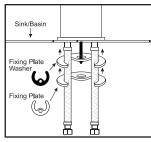
5. Position the fixing plate washer and fixing plate onto the bolt. The flexible hoses should be positioned towards the front of the sink/basin with the lever handle pointing towards the user. Fixing bolt positioned at the back.
