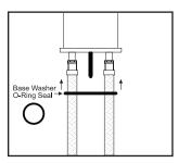
3. Place the base washer O-ring over the end of the hoses and insert into the base of the mixer.
