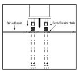
4. Feed the hoses through the sink/ basin hole, each end alternatively, and position the base washer between the sink/basin and the mixer base.
