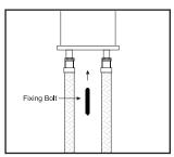
2. Screw the fixing bolt into the mixer base (remove fixing nut if installed).
