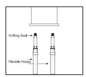
1. Firmly tighten the flexible hoses into the inlet tails at the base of the body. being careful to avoid damage to the O-ring seals. If the hoses have red and blue indicators make sure they are connected to the correct inlet port in the mixer.
