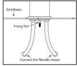
7. Connect the flexible hoses to the supply line, making sure the hot water is connected to the hot water
