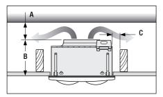
Fig. 3: Minimum clearances for installation
