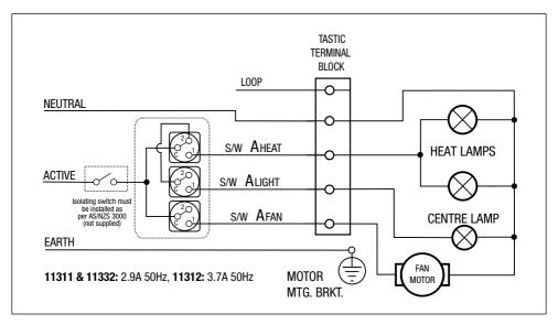
Fig. 7: Wiring diagram for model 11311,11312 and 11332. Centre lamp may be a CFL.
