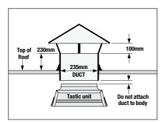
Fig. 5: Minimum external outlet requirements
