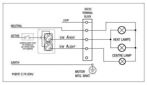
Fig. 8: Wiring diagram for model 11317. Centre lamp may be a CFL.
