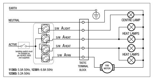
Fig. 6: Wiring diagram for model 11303, 12301 and 12303. Centre lamp may be a CFL.
