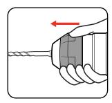
8 To remove the SDS<sup>+</sup> accessory pull back the locking sleeve and pull accessory out.
