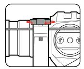
4 Drill the hole until the end of the depth rod touches the workpiece.
