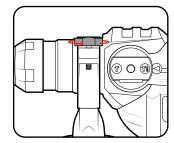
2 Adjust the depth rod so the drill bit extends beyond the end of the depth rod to the required drilling depth.
