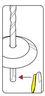
4 Press dust cover to the end of locking sleeve.
