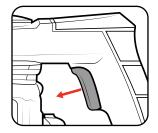
4 To start drilling squeeze the On/Off switch.
