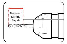
3 Tighten the depth rod securing nut to lock the depth rod into place.
