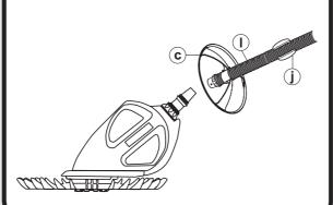
Before attaching the cleaner head, measure the suction flow at the hose the furthest away from the Skimmer box. Keep hose under water and connect the Pool Pulse to the hose using the Quick connector.
