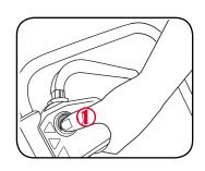
2. Pull the start/stop lever towards the handle to start the mower and then release the lock-off button.
