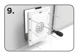
Screw into door from inside. Place nut over screw ends, cut off excess plastic screws. Optional: seal around frame of pet door with silicone.
