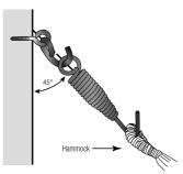
For sturdy masonry walls (not air/hollow/single brick or besser block) a 10mm dyna bolt with a large washer and rope can be used.
