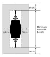
Allow a minimum of 50cm clearance range around the perimeter of your hammock when in use. <Fig.1>
