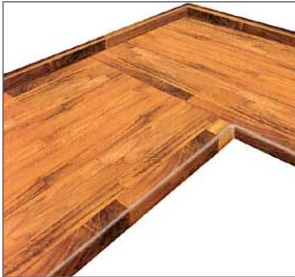
Fig. 17 Butt joint
