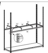
Place MDF board on bottom shelf to minimise buckling. Fix brackets 'B' so that top rivet sits on the upper legs and the bottom rivets sit on the lower legs. Repeat with brackets 'A', followed by braces 'G' as shown.
