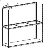
Fix brackets 'B' and 'A' to the top of legs 'D'.
