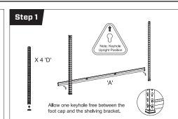
Place foot end caps onto the bottom of the legs 'D'. Note upright position. Place bracket 'A' onto the legs 'D'. A rubber mallet can be used to lightly tap all brackets into the keyholes on the legs.
