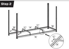
Use shelf bracket 'B' for the side brackets using the bracket 'A' from Step 1 as a guide for height. Use same shelving brackets for opposing sides as shown in the diagram. Place brace 'C' as shown.
