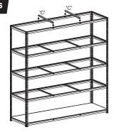
Fix remaining brackets to your desired height. Ensure that braces 'C' are fixed to all shelves.
